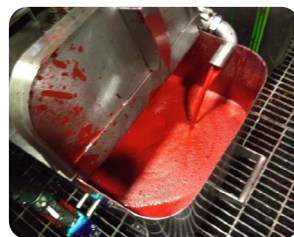
The ink is being "dropped" - into bucket adds air to the ink system
