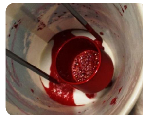
Micro Bubbles seen in the ink which can cause print issues
